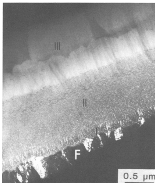
Figure 7 Dark-field image of the SCS coating on SiC filament (F) using \{111\} \beta SiC reflection. Small crystallites of SiC are present in regions I and II, while region III exhibits carbon growth features.
